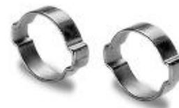
Hose or tubing with an internal diameter of less than 8mm and hose operated at a **pressure exceeding 50mbar** should always be secured by crimp clips or swaged fittings.
