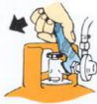
For butane cylinders with 'switch-on' or 'clip-on' connectors: Consult your dealer on the type of adaptor or regulator you require and fit in accordance with the manufacturer's instructions
