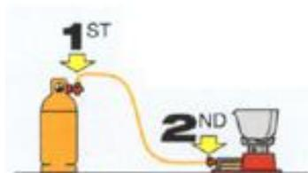
a) that the cylinder valve is closed first thus allowing the gas in the system to burn off;
