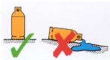
Make sure the cylinder is large enough for your requirements. Cylinders must be sited away from any heat source, in a well-ventilated place and must stand in a stable upright position.
